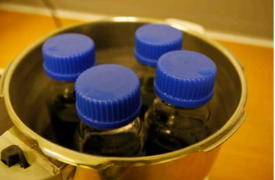
Make sure that the pressure is released before opening the lid. Caution! The bottles are incredibly hot. After the bottles cooled down a bit the caps can be closed.
