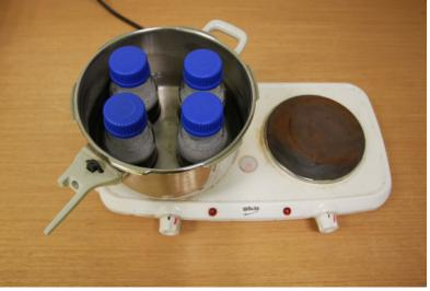
Shake the bottles well, until the ingredients have dissolved in the distilled water. The caps of the laboratory bottles must be slightly unscrewed so that the pressure can escape. Fill the pressure cooker a bit with water (about one third of the pots volume).
